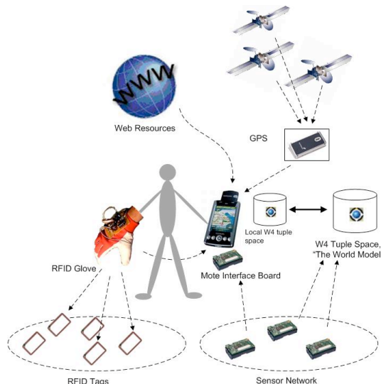
Figure 4: User equipped with a PDA and pervasive devices can acquire contextual information from the physical world. Sensed data are integrated in W4 atoms with information coming from the Web, and stored both in local and global W4 tuple spaces.
