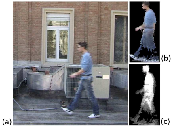
Figure 5: An example of appearance-based tracking showing: the input image (a), the appearance mask model AMM (b), and the probability mask PM (c).
